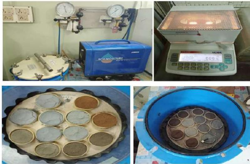
Fig. 1. Pressure Plate Apparatus
