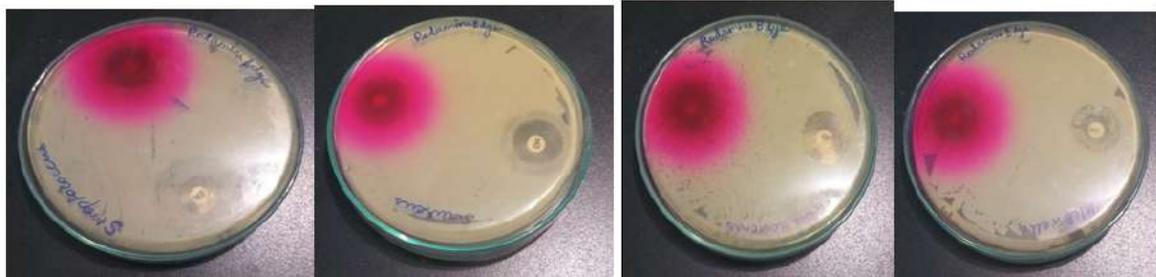
Figure 13. The inhibition area diameter of RBMO nanoparticles
